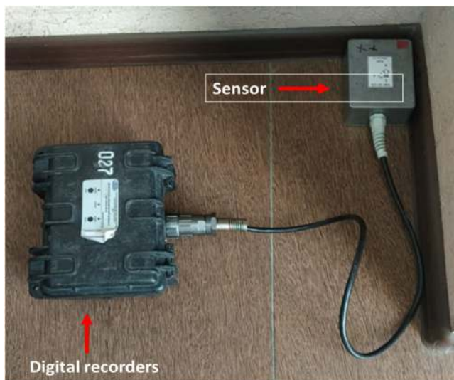
Fig. 6. The recording process on the first floor of the surveyed structure using the Baikal-7 recorder and a three-component GD-10 sensor.
